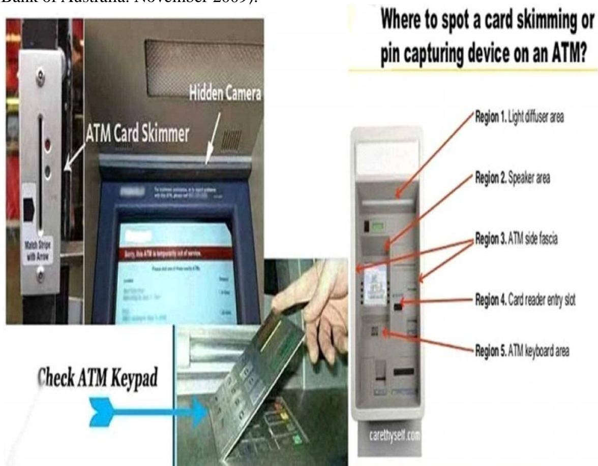
Fig.2. ATM skimming devices & ATM's different regions.
